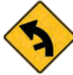
SIDE ROAD JUNCTION ON A CURVE
