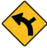
SIDE ROAD JUNCTION ON A CURVE
