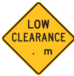
LOW CLEARANCE ...m (AHEAD) W4-8B W4-8C
