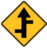
STAGGERED SIDE ROAD JUNCTION
