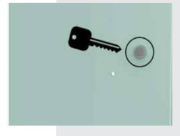
• While pushing the override with the tool, use the key to rotate the CAM to open the door
