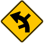
SUCCESSIVE SIDE ROAD JUNCTION
