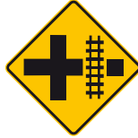
TRAIN CROSSING INTERSECTION
