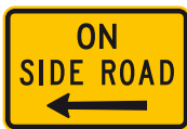
ON SIDE ROAD W8-3A 600 x 400 W8-3B 750 x 500 W8-3C 900 x 600 (L or R)
