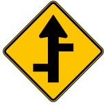
STAGGERED SIDE ROAD JUNCTION
