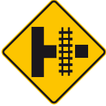
TRAIN CROSSING T-JUNCTION
