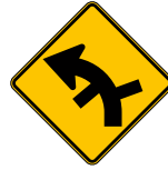
SUCCESSIVE SIDE ROAD JUNCTION
