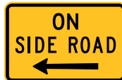
ON SIDE ROAD W8-3A 600 x 400 W8-3B 750 x 500 W8-3C 900 x 600 (L or R)
